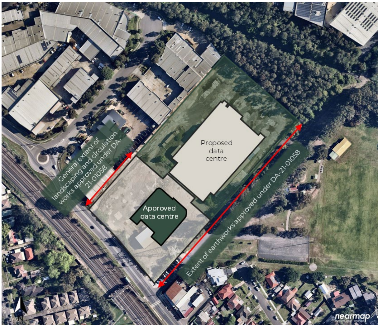
Figure 17: Illustrative figure showing approved and proposed development Source: Nearmap modified by Patch
