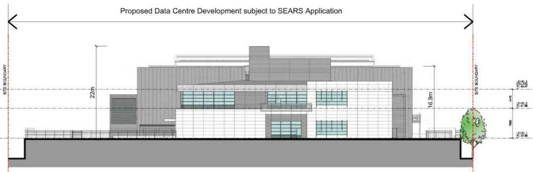
1 SOUTH-WEST ELEVATION SCALE 1:250
