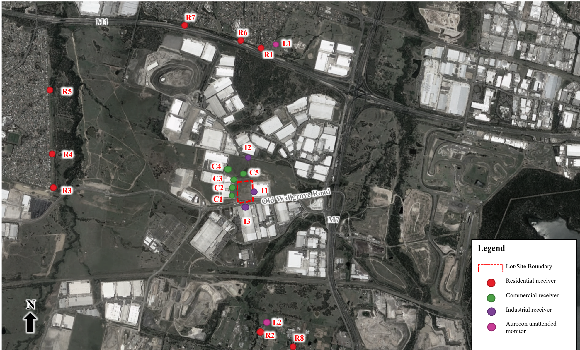
Figure 3: Site, sensitive receivers and noise monitoring locations
