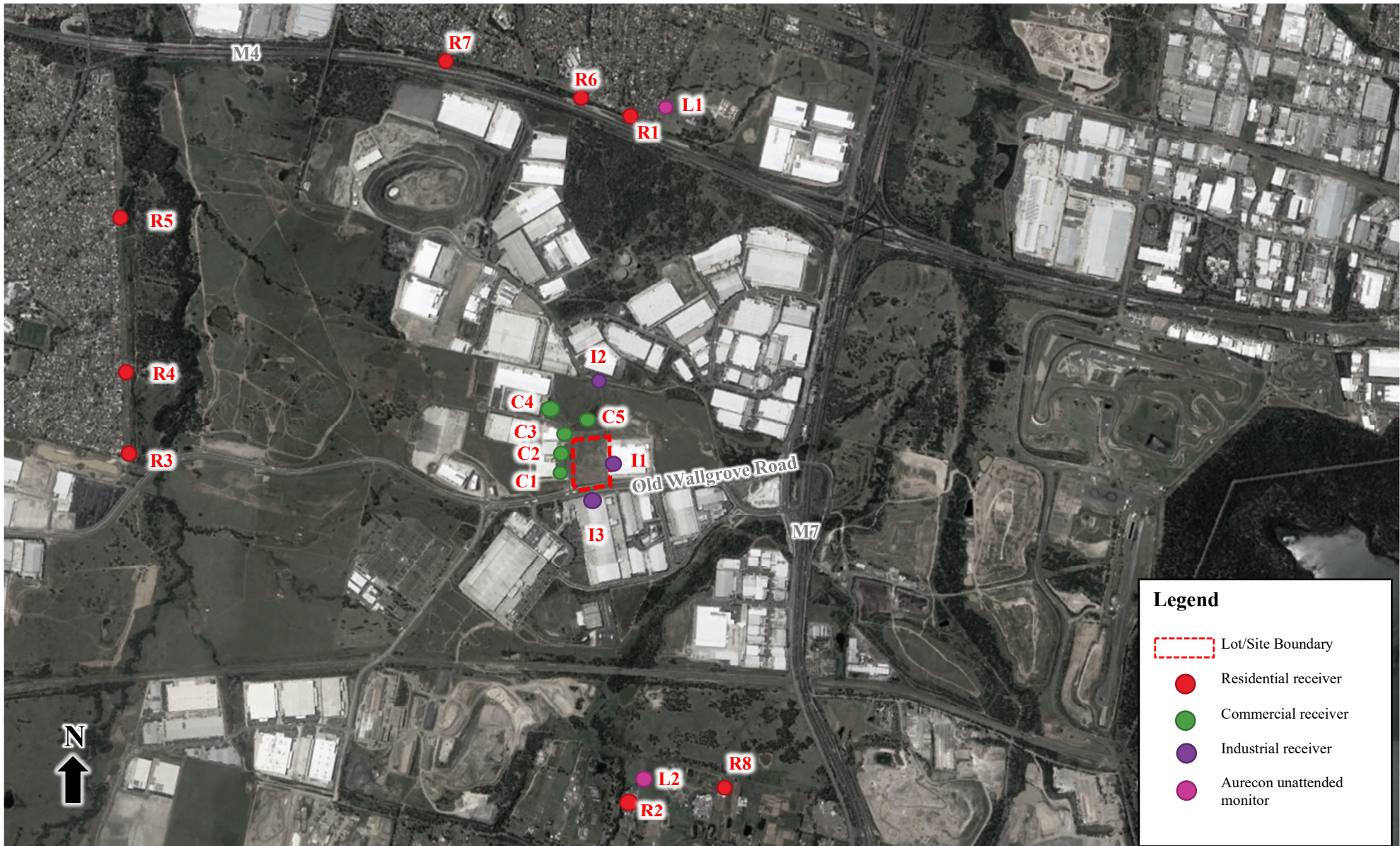
Figure 3: Site, sensitive receivers and noise monitoring locations
