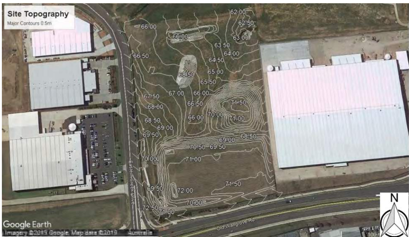
Figure 13 – Site topography (Crux Surveying Australia, 2019) superposed on satellite image (Google Maps, 2019)
