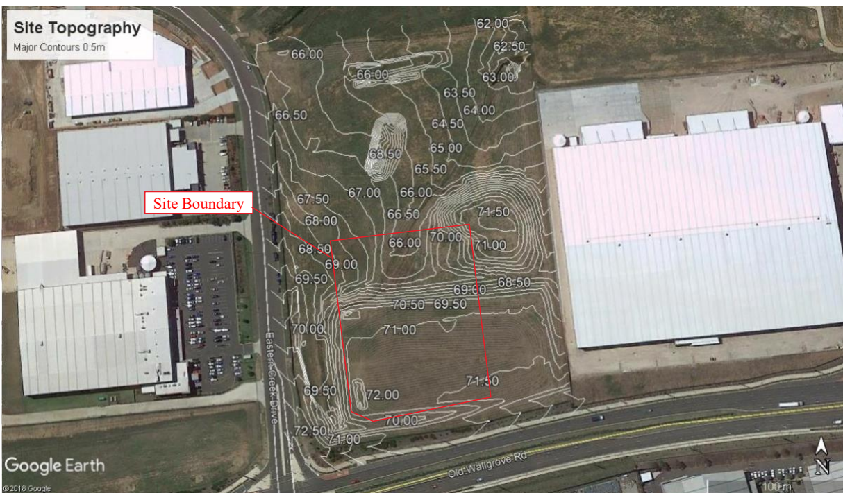
Figure 11 Pre-construction site topography (Crux Surveying Australia, 2019) superposed on satellite image [2]
